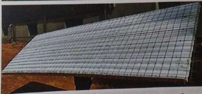
Factory-made EPS core panel and welded wire mesh reinforcement
