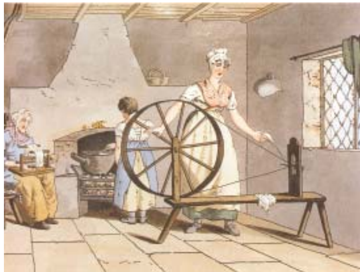
Fig. 3 – Spinning in the eighteenth century. You can see each member of the family involved in the production of yarn. Notice that one wheel is moving only one spindle.
