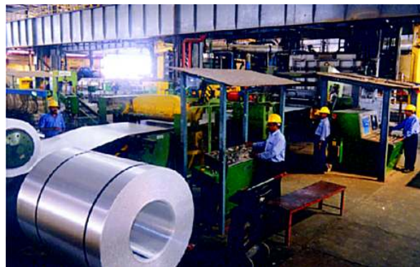
Fig. 6.6: Strip casting mill at smelter of NALCO
