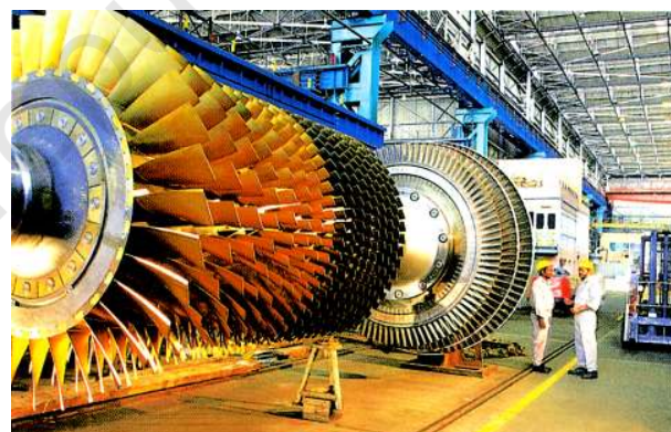
Fig. 6.10: Gas turbine rotor an assembly bed at BHEL, Hyderabad
