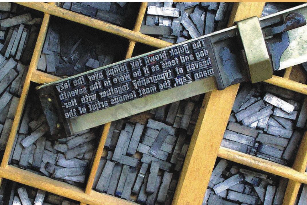
Lead type in compositor trays; (inset) type arranged and fixed in a temporary frame
